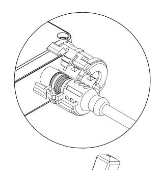
TO INSTALL LOCKOUT DEVICE, PLACE AROUND CORDSET END AND CLOSE UNTIL CONNECTOR SNAPS CLOSED. REFERENCE DIAGRAM OF CONNECTOR.
